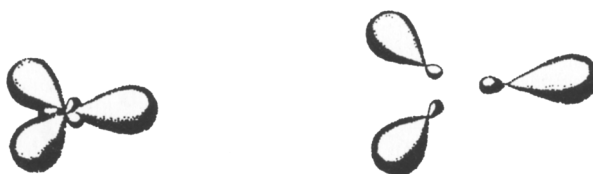
Fig. 24.13. Left: The density distributions of the three electrons in the case of trigonal ( sp^2 -) hybridisation of carbon. Right: Exploded view
