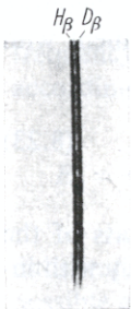
Fig. 8.6. \beta lines of the Balmer series in a mixture of equal parts hydrogen ( 1 H) and deuterium ( 2 H). One sees the isotope effect, which is explained by motion of the nucleus. The lines are about 1 Å apart and have the same intensity here, because the two isotopes are present in equal amounts [from K. H. Hellwege: Einführung in die Physik der Atome , Heidelberger Taschenbücher, Vol. 2, 4th ed. (Springer, Berlin, Heidelberg, New York 1974) Fig. 40a]
