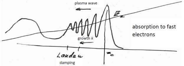
At higher intensities plasma wave damps via nonlinear mechanism of wavebreaking – energy is transferred to a small group of so called ,,hot (fast) electrons. Electrons are accelerated both into target, and to plasma-vacuum, where most of electrons are reflected in electrostatic field of sheath back into target.
