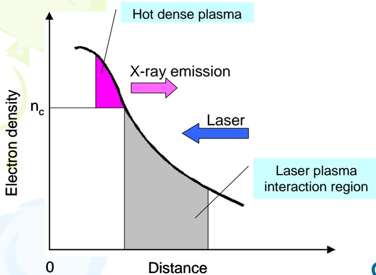
EUV radiation is emitted from hot dense plasma near the electron critical density  $n_c$ .
