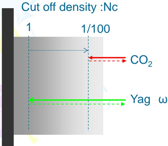
CO<sub>2</sub> laser light is absorbed by low density plasma. Thermal boiling of liquid Sn is avoided.
