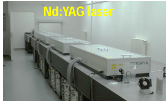
Laser plasma EUV source driven by a 10 J/10 ns/10 Hz Nd:YAG laser
