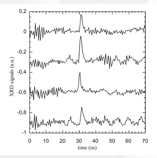
Temporal evolution of laser emission obtained in four consequence pulses. The jitter of the laser spike is ~ 1 ns.
