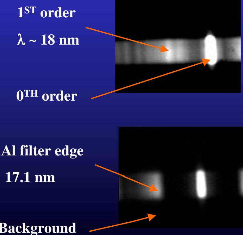
0.75  $\mu\text{m}$  Al foil filter transmittance
