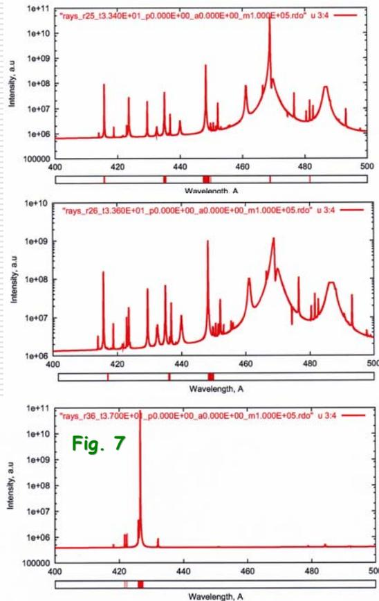
Evaluated spectra forecast also strong **lasing with the wavelength  $\lambda = 42.6$  nm at  $t = 37$  ns**, when  $T_e = 105$  eV, and  $N_e = 3.14 \cdot 10^{18} \text{ cm}^{-3}$ .
