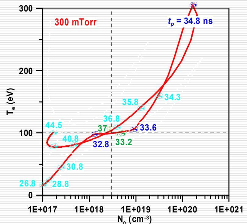
Fig. 8 : Diagram of electron temperature  $T_e$  and density  $N_e$ , labels denote time in ns
