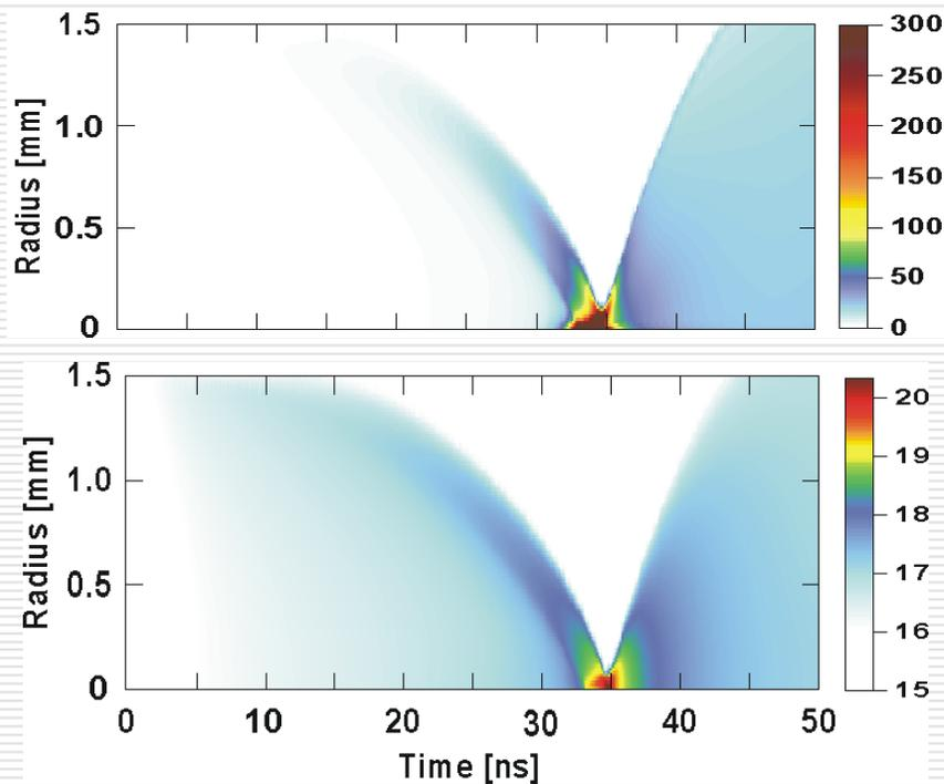
Resulting peak values of plasma electron temperature and density on the axis are  $T_{e,max} \cong 300 \text{ eV}$  and  $N_e \cong 10^{20} \text{ cm}^{-3}$ .
