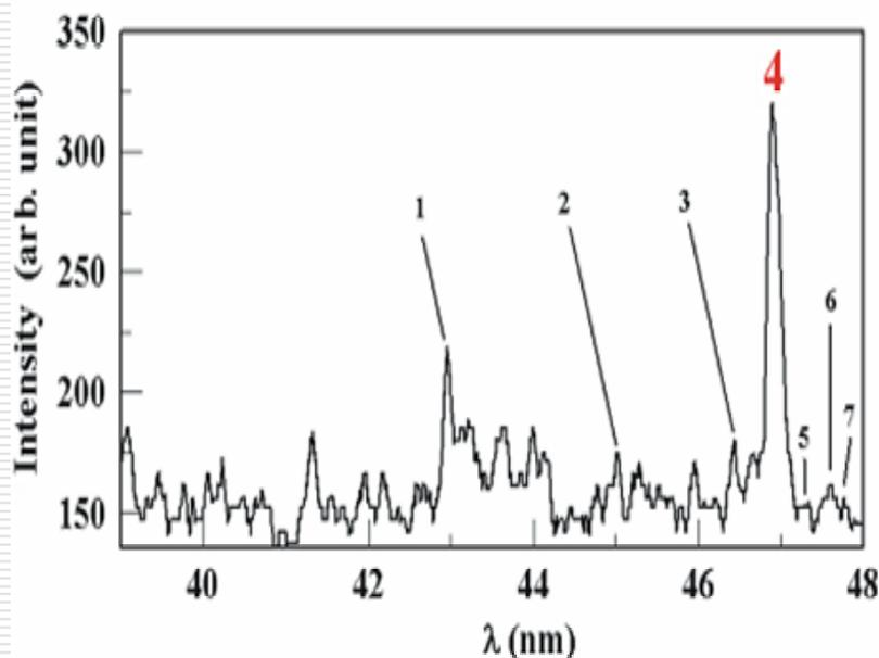
Fig. 3 : Measured time integrated spectrum ( $2R_0=3$  mm,  $p_0 = 300$  mTorr,  $I_{max} = 22.5$  kA)
