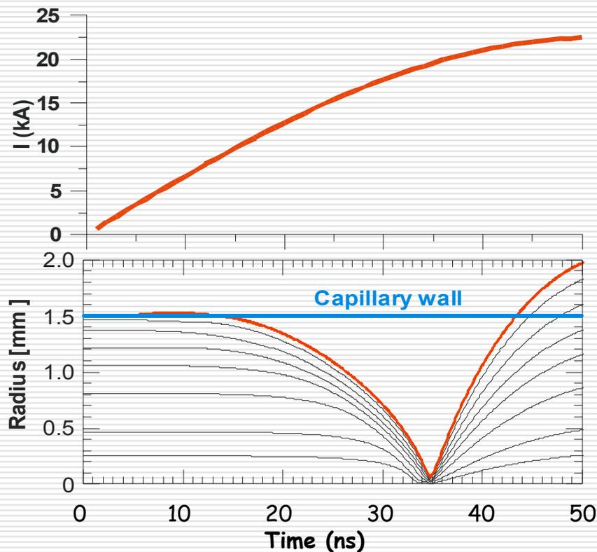
Capillary discharge plasma quantities have been evaluated by means of **the NPINCH code** under 1-dimensional 2-temperature, 1-fluid MHD approximation
