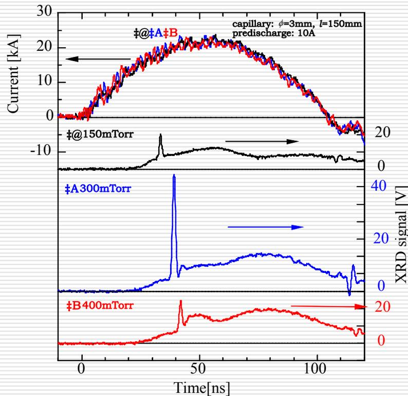
**Fig. 1** : (a) Electric current, (b), (c) and (d) X - ray signals for various argon pressures
