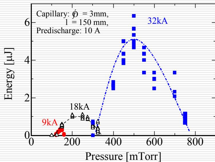
Fig. 2 : Pressure dependence of the output X - ray energy for various peak currents
