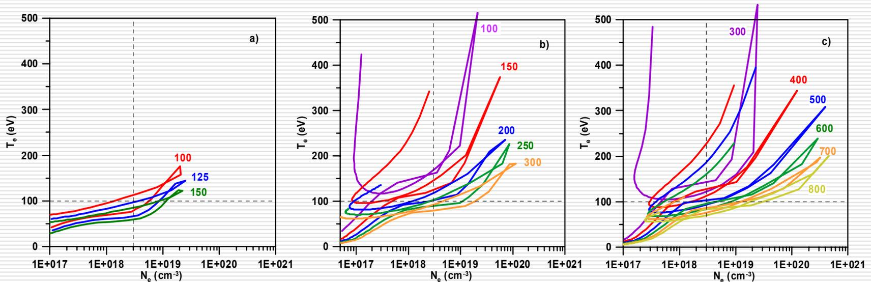
**Fig. 9** : Pinch plasma evolution in phase-space  $N_e - T_e$  for  $d_0 = 3 \text{ mm}$  and various filling pressures; a)  $I_{max} = 9 \text{ kA}$ , b)  $I_{max} = 18 \text{ kA}$ , c)  $I_{max} = 32 \text{ kA}$
