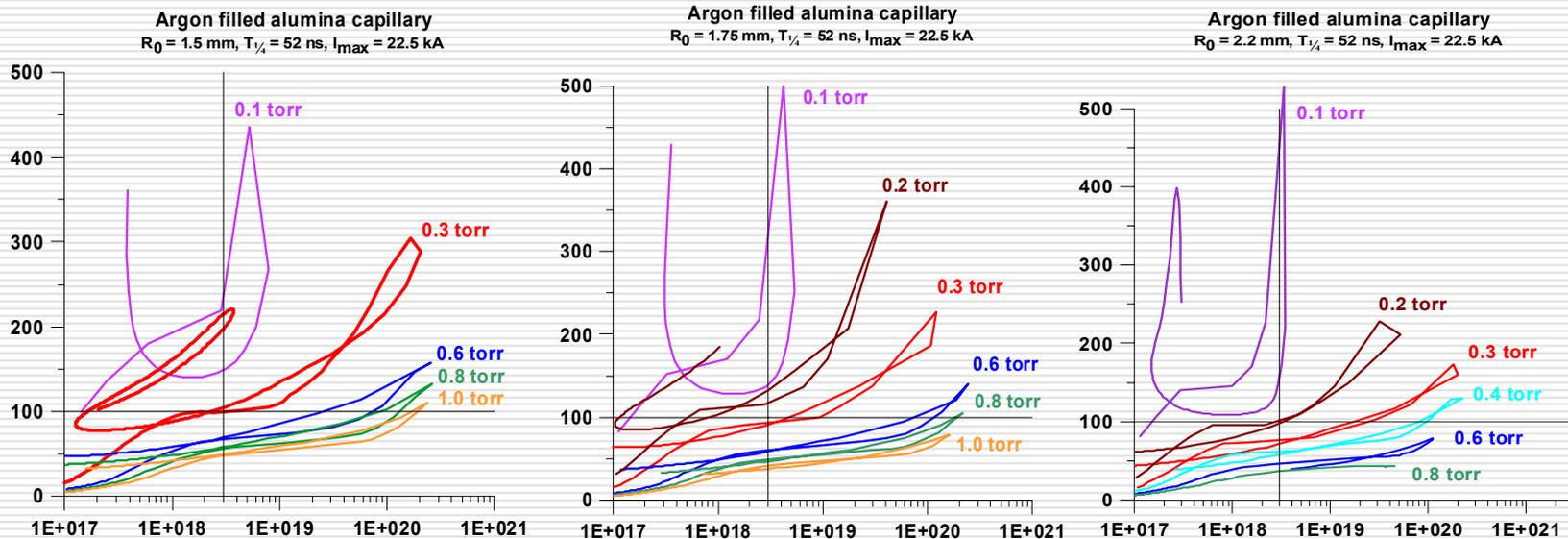
Fig. 10 : Pinch plasma evolution in  $N_e$ - $T_e$  space a)  $2R_0 = 3$  mm, b)  $2R_0 = 3.5$  mm, c)  $2R_0 = 4.4$  mm
