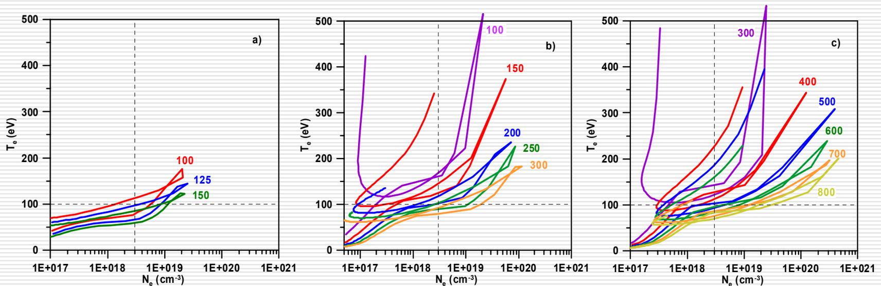
Fig. 9 : Pinch plasma evolution in phase-space  $N_e - T_e$  for  $d_0 = 3 \text{ mm}$  and various filling pressures; a)  $I_{max} = 9 \text{ kA}$ , b)  $I_{max} = 18 \text{ kA}$ , c)  $I_{max} = 32 \text{ kA}$
