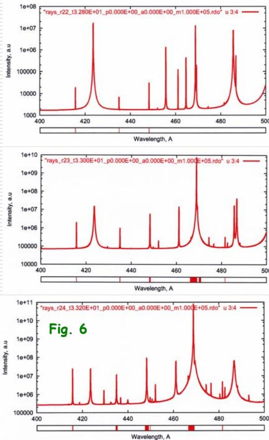
Calculated instantaneous spectra of Ar plasma radiation at selected time moments demonstrate quick changes of structure around the time when  $\langle Z \rangle \cong 8$ . On the bars below the spectrum plots regions where radiation is amplified are indicated. The strongest lasing occur on transition  $2p5\ 3s\ ^1P_1 - 2p5\ 3p\ ^1S_0$  in Ne-like argon.
