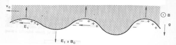
Due to ion motion, charge is formed at the rippled surface, it induces electric field, and it causes E×B drift of ions and electrons that enhances ripples Derivation from 2-fluid description (derivation is also possible from MHD):
