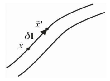
and velocity  $\vec{u}'$  in point  $\vec{x}'$  is  $\vec{u}' = \vec{u} + (\delta \vec{l} \nabla) \vec{u}$ , then time derivative of the element  $\frac{\mathrm{d}}{\mathrm{d}t} \delta \vec{l} = \vec{u}' - \vec{u} = (\delta \vec{l} \nabla) \vec{u}$ .
